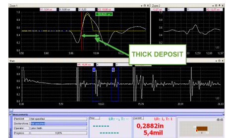
Figure 5. Graphic displays of the ultrasonic wave shape allow Valmet operators to accurately present the scale thicknesses in a comprehensive report.
